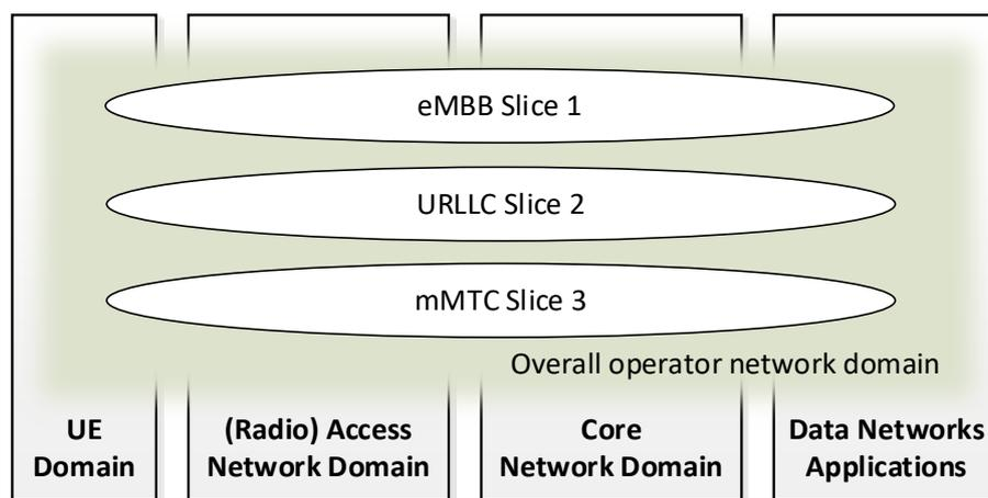
*Figure 4: Network slicing concept with three slice types.*
