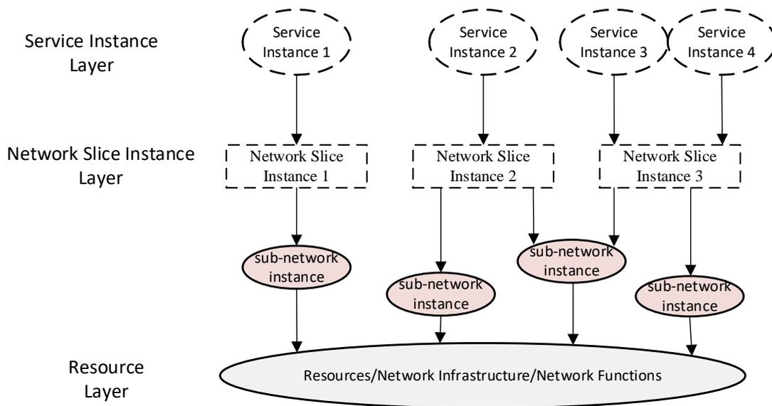
**Figure 6:** Network slicing concept with sub-network instances.
